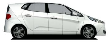
Figure 4-1 Global Vehicle Target (GVT)
