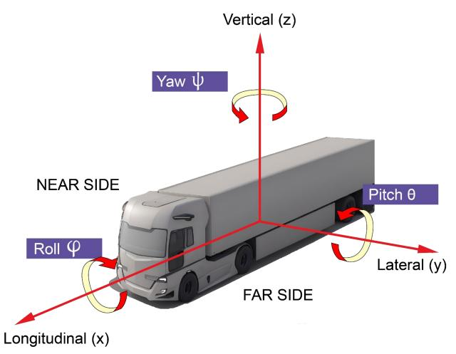
Figure 3-1 Coordinate system and notation
