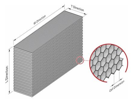
Figure 3 Aluminium Honeycomb Orientation
