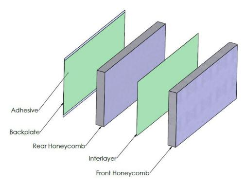
Figure 1: Exploded Isometric View
