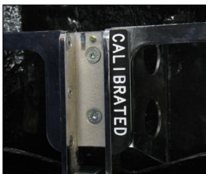
Figure 30: Calibrated Torso angle measurement surface block attached to trunk of weight hanger arm.
