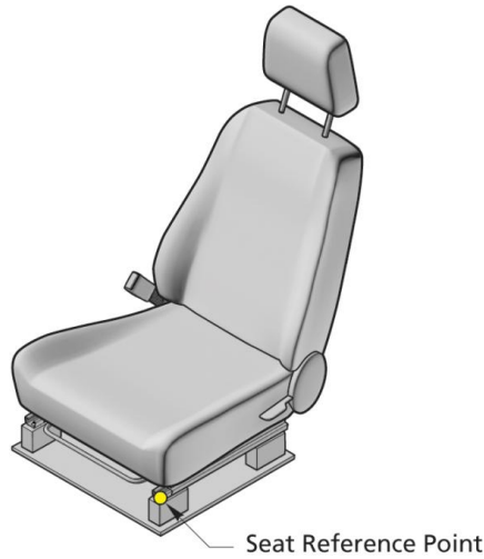
Figure 1: Definition of the Seat reference point.
