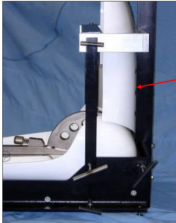
Figure 28: HPM installed into the jig. A check should be made to ensure that the gap between the HPM back pan and jig vertical support is no more than 4mm.
