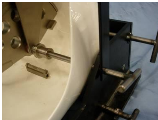
Figure 25: H-Point locator bars installed through vertical support rods, jig side and HPM H-Point location.
