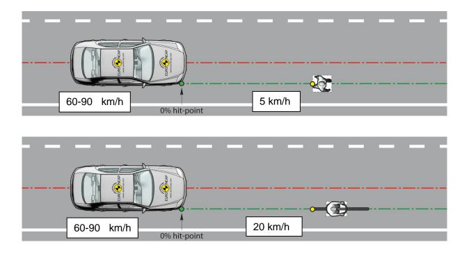
A valid test run shall be considered when the 0% impact location is achieved with a lateral offset accuracy of + 10cm - 0cm.
