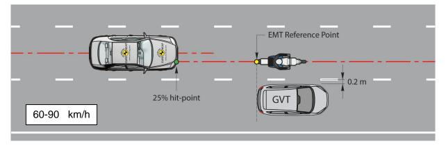
b) A stationary GVT positioned centred in-lane and 1m in front of the EMT:
