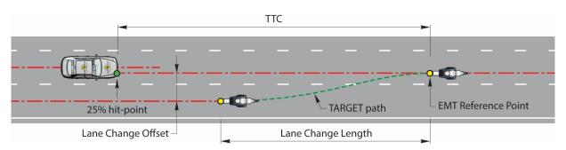
To ensure a realistic trajectory and sufficient repeatability/reproducibility across different EMT platforms, the following EMT boundary conditions shall be met during the Lane Change length:
