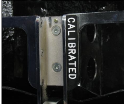
Figure 30: Calibrated Torso angle measurement surface block attached to trunk of weight hanger arm.
