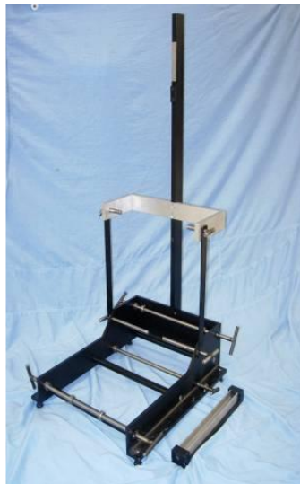
Figure 24: HPM Calibration Jig (GLORIA)
