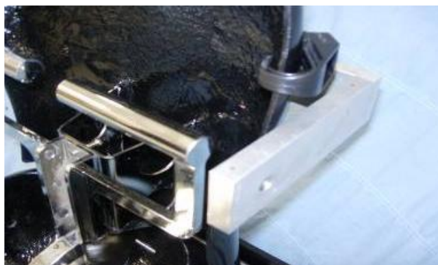
Figure 26: HPM back pan held by retaining strap.
