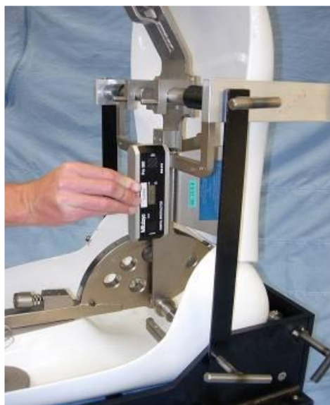
Figure 29: Measurement being taken of the torso angle at the weight hanger trunk by a digital inclinometer.
